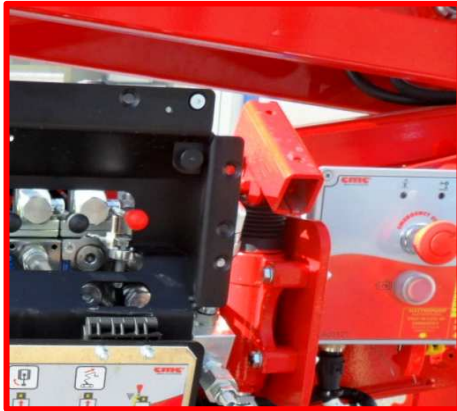
Picture 18: insert for manual pump.
