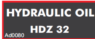
Picture 45: indication for oil refill.
