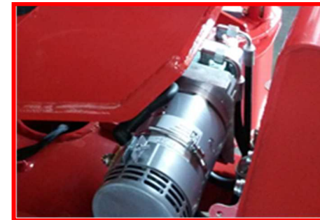
Picture 21: emergency electropump (*optional).
