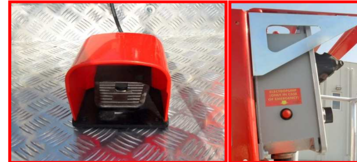
Picture 10: “dead man” pedal (*optional) and left side of basket control station.
